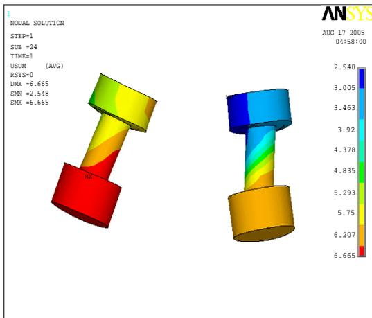
Figure 12 Deformation of bolts in specimen 1
