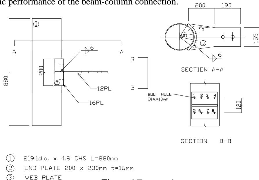
**Figure 1** Test specimen
