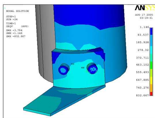
Figure 15 Von Mises stress of specimen 3
