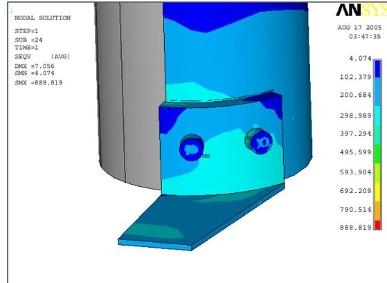
**Figure 11** Von Mises stress of specimen 1
