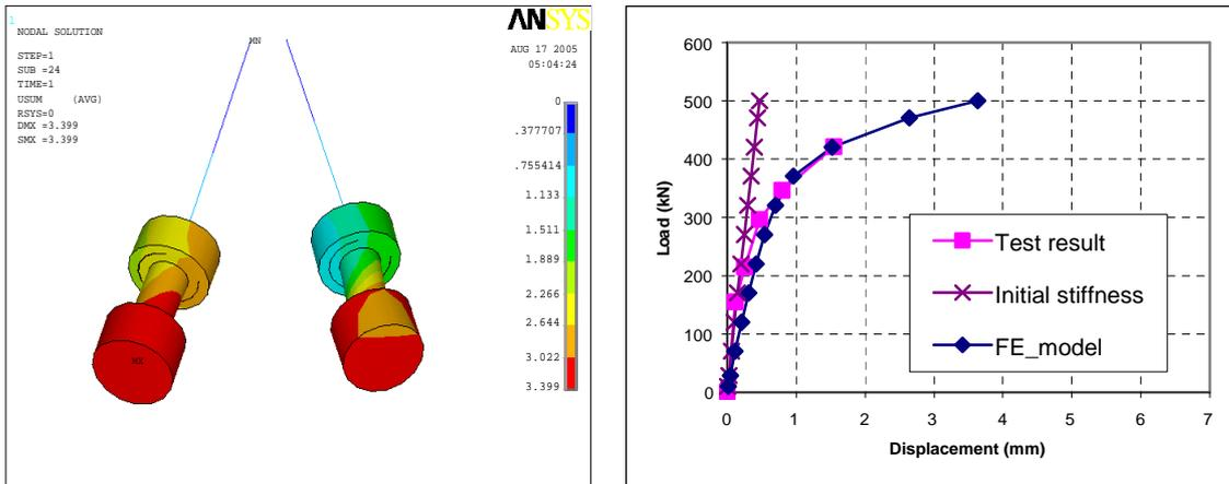
**Figure 16** Deformation of bolts and extensions **Figure 17** Load-displacement of Specimen 3
