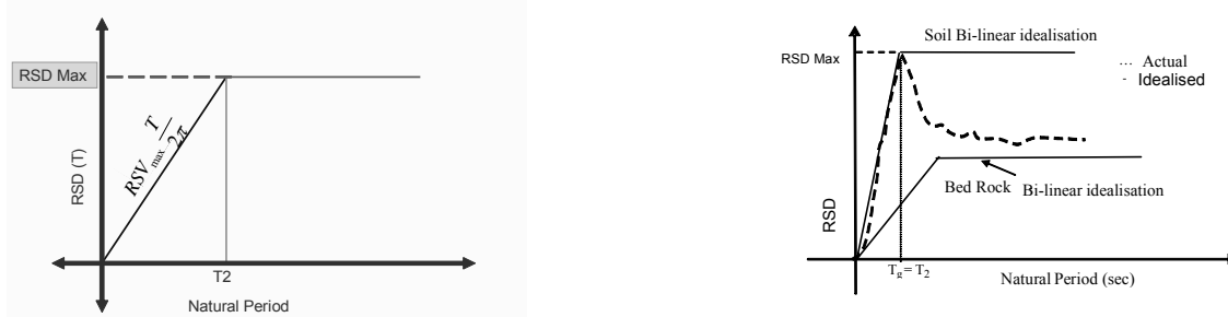
(a) Simplified displacement response spectrum on rock site (b) Simplified displacement response spectrum on soil site Figure 6. Simplified displacement response spectrum.
