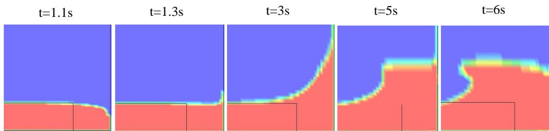
Figure 5 Tsunami wave runup on a rigid wall
