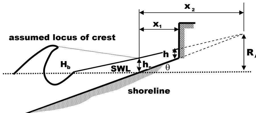
Figure 2 Wave pressures from broken waves on walls landward of the still-water line
