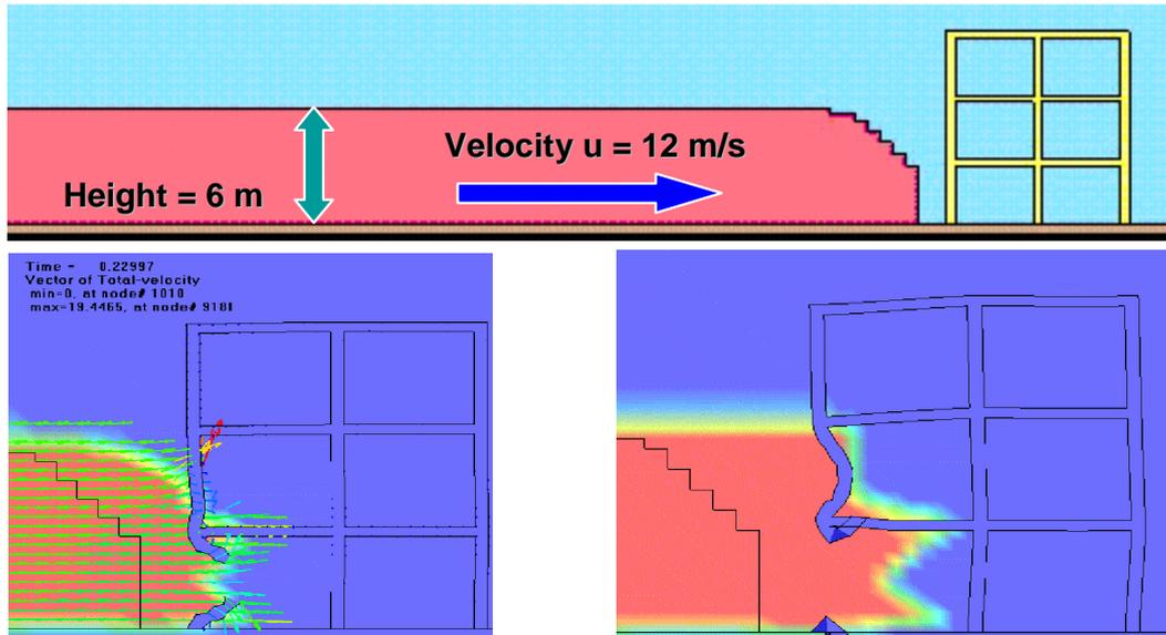
Figure 7 Structural damage due to a Tsunami wave
