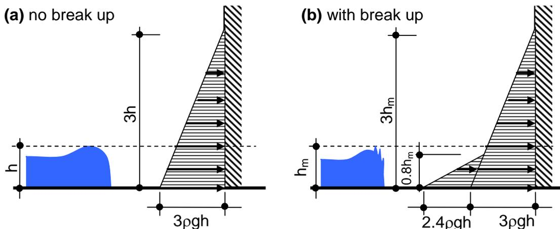
Figure 1 Tsunami wave pressure distribution with/without soliton break-up
