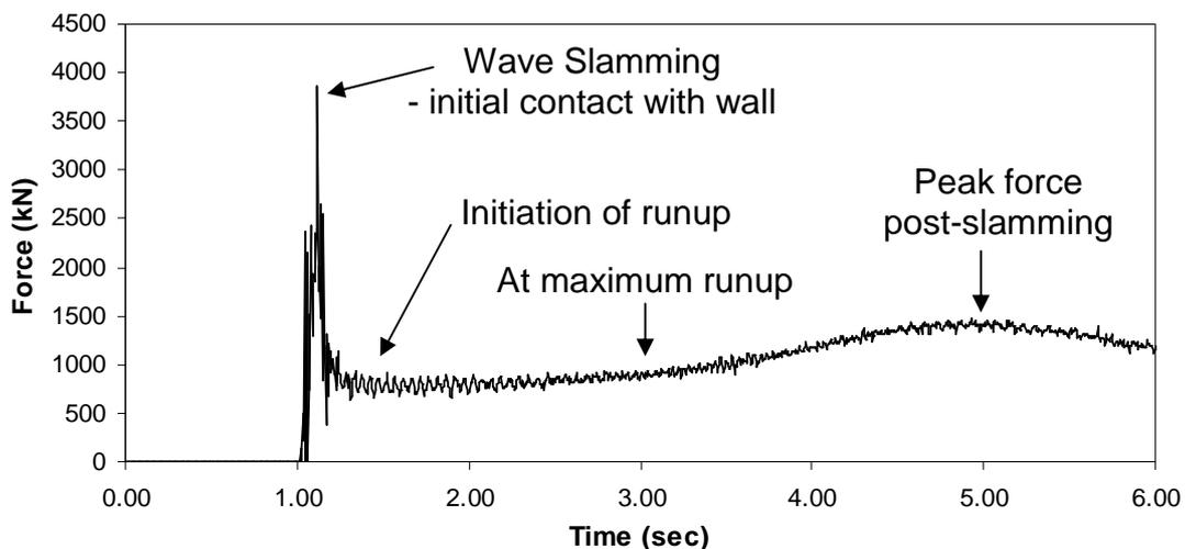
Figure 6 Tsunami force on a rigid wall
