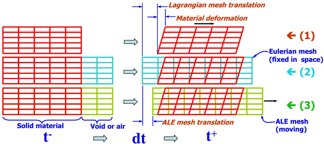
Figure 3 Description of Arbitrary Lagrange Euler (ALE) technique used in LS-DYNA
