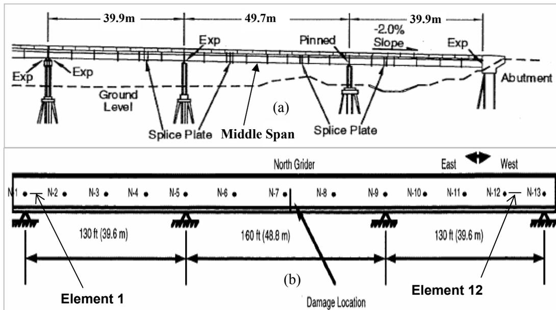
Fig. 1. Locations of the SET1 accelerometers during the FVTs: (a) portion of the I-40 Bridge tested; (b) north plate girder with location of damage and accelerometers indicated.
