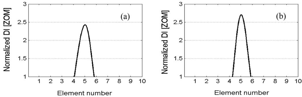
Fig. 5.2. Damage localization results from normalized ZOM of the wavelet spectra using SET2 data: (a) damage scenario E-3; (b) damage scenario E-4.
