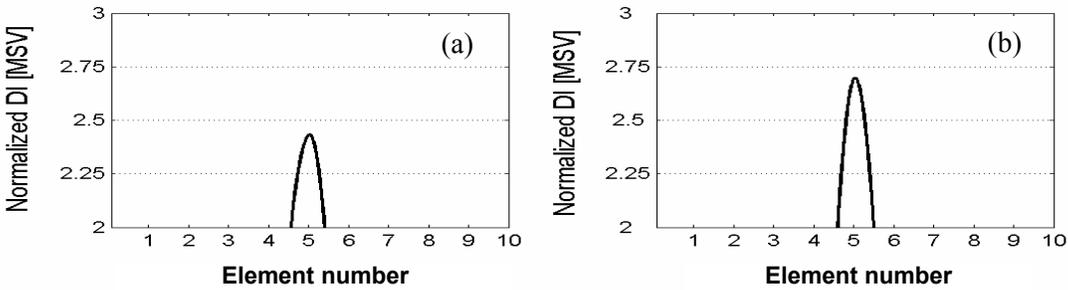
Fig. 3.2 Damage identification results from normalized MSV of response of the I-40 Bridge using SET2 modal data: (a) damage scenario E-3; (b) damage scenario E-4.
