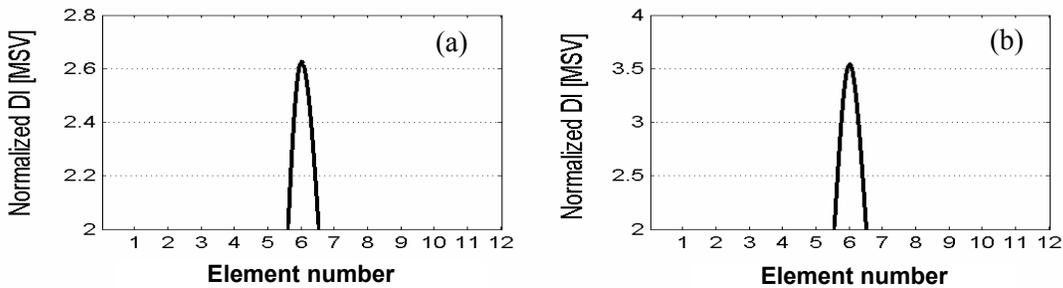
Fig. 3.1 Damage identification results from normalized MSV of response of the I-40 Bridge using SET1 modal data: (a) damage scenario E-3; (b) damage scenario E-4.
