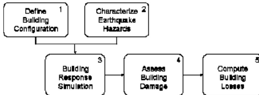
**Figure 1** Proposed procedure for seismic loss assessment (ATC, 2007)
