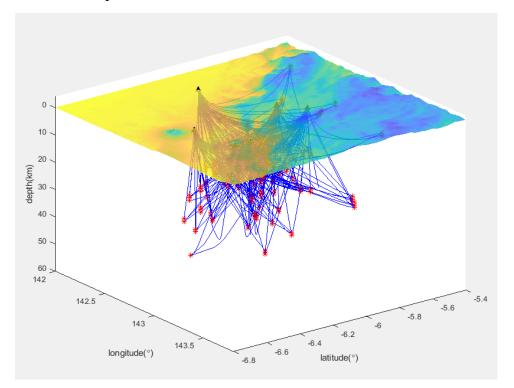
Figure 6: The ray paths and the coverage for the events and the receivers over the topography of the study area (earthquakes-red stars, stations-black triangles, ray paths-blue lines).
