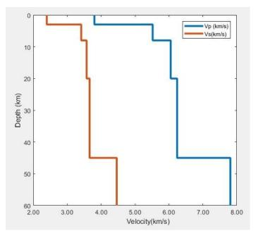
Figure 5: Initial velocity model utilised for the Southern Highlands of PNG
