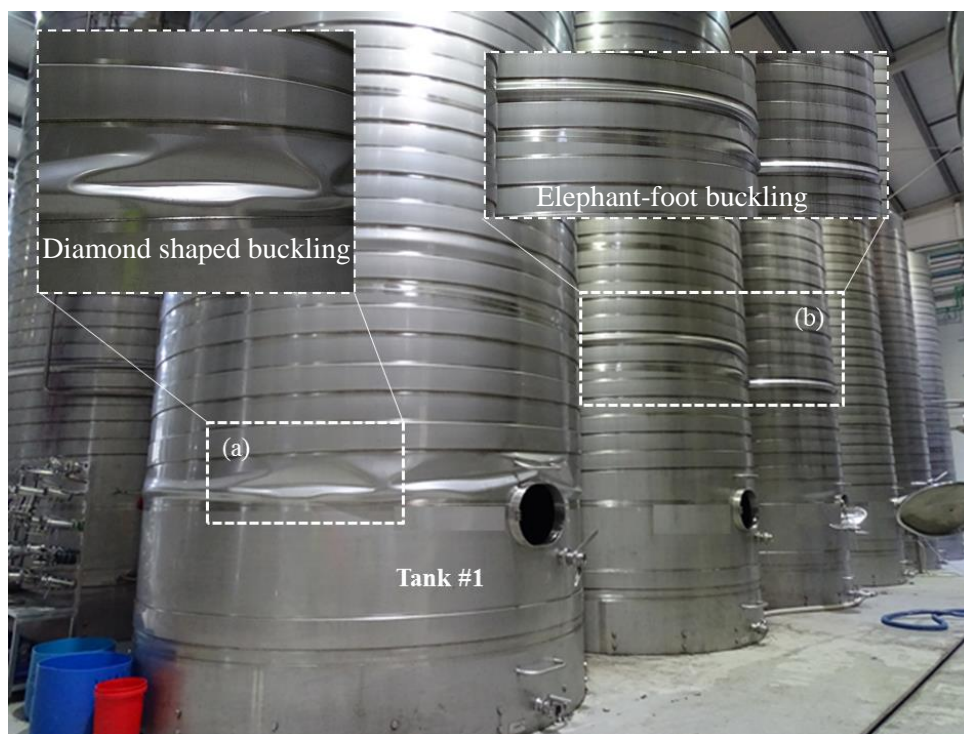
Figure 2. Example of buckling in flat-based tanks (capacity of 100 kL): (a) diamond shaped buckling; (b) elephant-foot buckling
