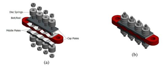
Figure 1: (a) components of the RSFJ (b) RSFJ assembly
