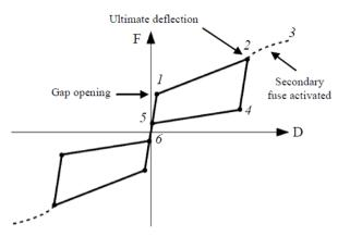
Figure 4: The flag-shape response of the RSFJ including the effect of the collapse-prevention secondary-fuse mechanism [13]
