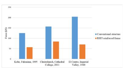
Figure 8: Comparison of maximum base shears under scaled earthquakes
