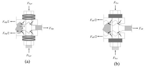
Figure 3: Free body diagram of the RSFJ at (a) slip state (b) ultimate state [11]
