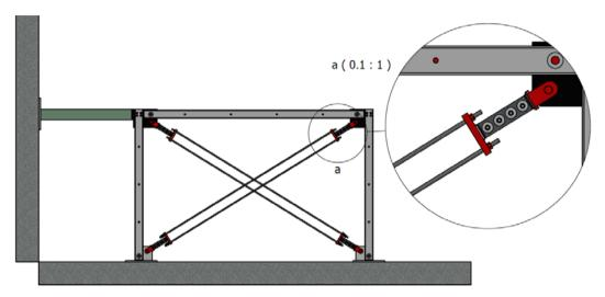
Figure 6: Designed test set-up: (a) details of the tension-only connection
