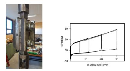
Figure 5: Joint component testing of the RSFJ [11]
