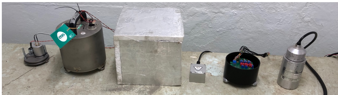
Sensors (l-r): 4.5Hz and 2Hz passive geophones (on circular plate), 1Hz active seismometer, optical sensor under foam box, LF boosted 10Hz & 4.5Hz geophones, and 1Hz passive geophone
