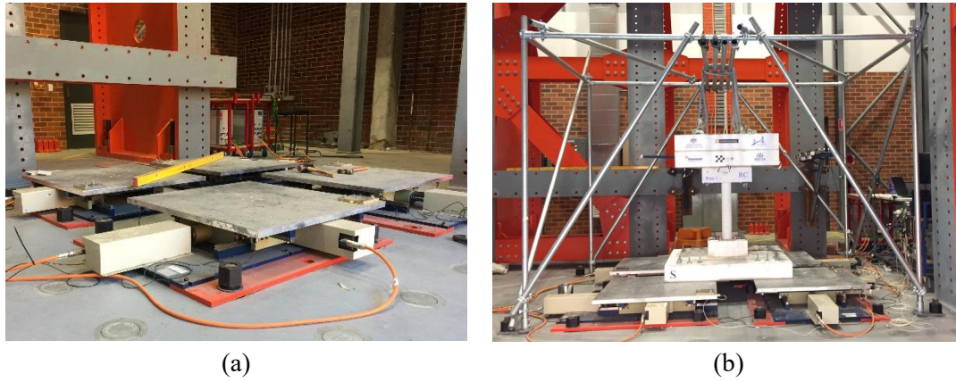
Fig. 2. (a) Shake table arrangement, (b) test setup
