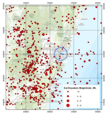
**Figure 1**. Recorded earthquake activity in the Sydney Basin. The schematic location of the tunnel alignments is shown as a blue line. The blue circle represents a distance of 20 km from the alignment.
