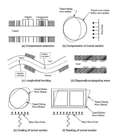
Figure 2. Deformation modes of tunnels due to seismic waves (Hashash et al., 2011).
