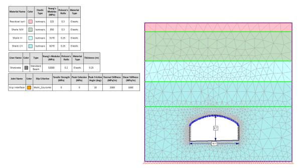
Figure 3. Example of model geometry used for numerical analysis of racking deformation.
