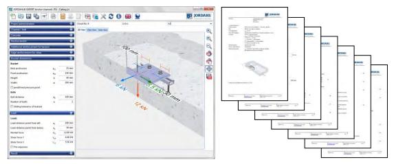
Figure 6. Screenshot of the graphical user interface of a professional anchor channelchannel bolt design software and the print of analysis ready for the checking engineer.
