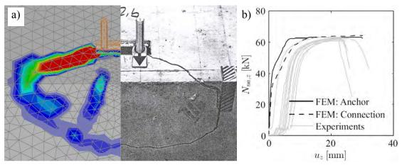
Figure 5. a) Example numerical simulation of experimental test (Potthof (2008)); b) Example load-displacement curves of simulations and tests (Kocur et al. (2016)).
