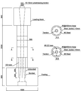
Fig. 1 Design details of the simulated column (Chou et al. 2013)
