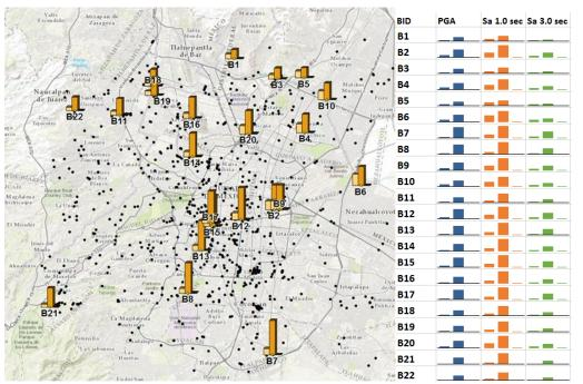
Figure 2 Estimated ground motion exposure in Mexico City for the three earthquake events
