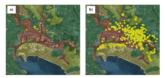
Figure 7 Damage distribution (Collapse Prevention) for (a) 500-year and (b) 2500-year return period earthquakes
