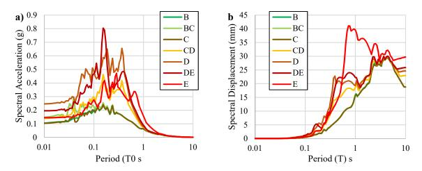
Figure 4 500-year return period spectra (a) acceleration response and (b) displacement response acceleration response
