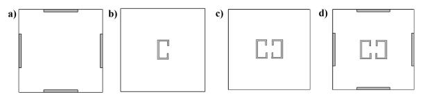
Figure 6 The different idealised building configurations used for RC buildings in Australia (a) Type 1 (b) Type 2 (c) Type 3 and (d) Type 4
