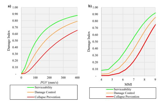
Figure 8 Fragility curve results for LR RC structural wall buildings for an intensity measure of (a) *PGV* and (b) MMI
