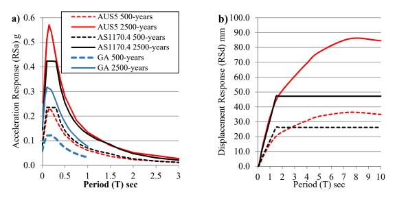
Figure 1 (a) acceleration and (b) displacement response spectra for Melbourne
