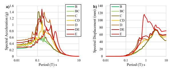
Figure 5 2500-year return period spectra (a) acceleration response and (b) displacement response acceleration response
