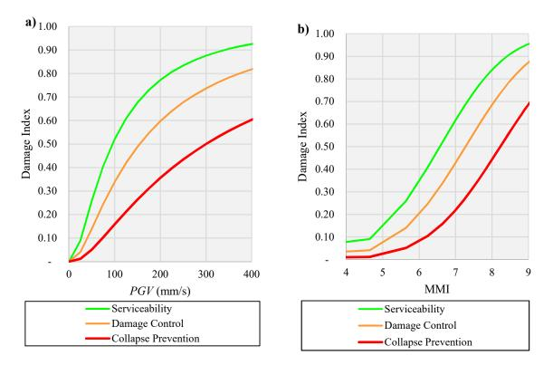
Figure 9 Fragility curve results for MR RC structural wall buildings for an intensity measure of (a) *PGV* and (b) MMI
