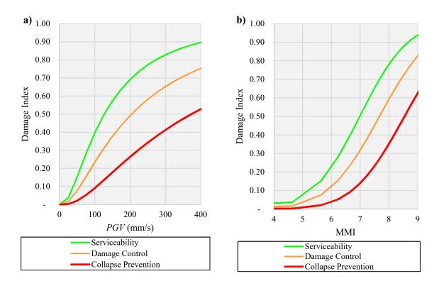
Figure 10 Fragility curve results for HR RC structural wall buildings for an intensity measure of (a) *PGV* and (b) MMI
