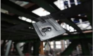
Figure 15. Failure of hanger wire
