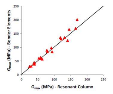
Fig.5 Comparison of small-strain shear modulus of recycled concrete aggregate between resonant column and bender element tests
