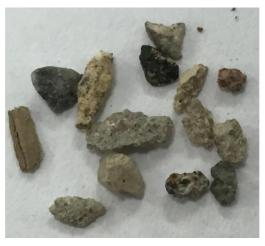
Fig.1 Image of recycled concrete aggregate fraction 1.18-2.36 mm used in the study
