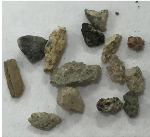
Fig.1 Image of recycled concrete aggregate fraction 1.18-2.36 mm used in the study
