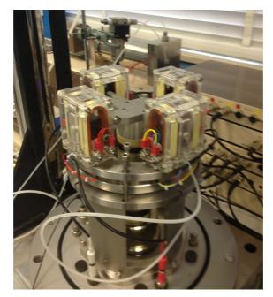
Fig.2 The Stokoe-type resonant column of UNSW Australia
