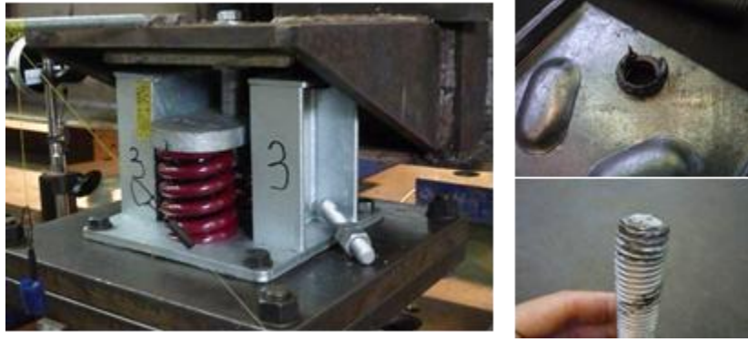
Figure 5. Failure modes of tested restrained isolators
