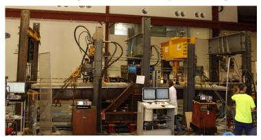
Figure 6: Large sub-assemblage test for composite frame with blind bolts
