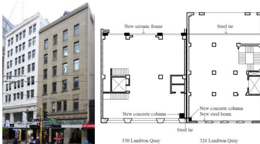
Figure 1: 326 and 330 Lambton Quay: tied together as part of the strengthening strategy
