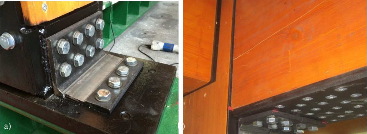
Figure 8: a) Fracture of dissipative angles at base and b) tension cracking of beam at first floor
