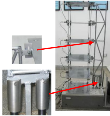
Figure 6 Setup of the frame and damper
