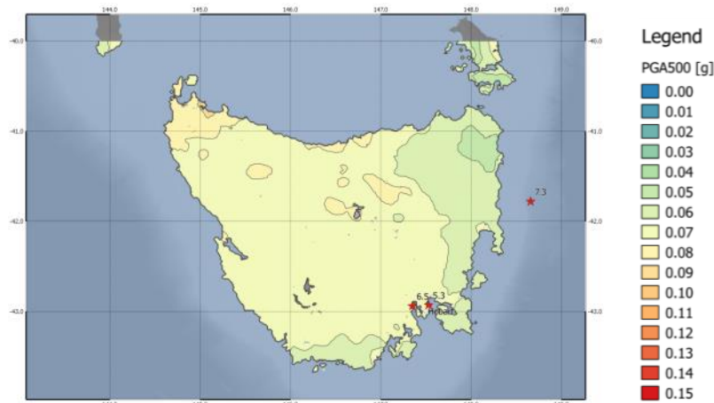
Figure 6: Plot of the mean 500-year exceedance PGA around Hobart on a 1x1 km grid in g=9.81 \text{ m/s}^2 .
