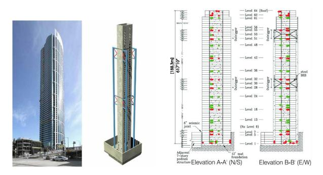
*Figure 1.* (Left) Picture of One Rincon Tower and its core skeleton with outrigger columns and attachment of BRB's to the core. (Right) Vertical sections of the building showing locations of the accelerometers along the height of the building (<u>www.stongmotioncenter.org</u>, last visited July 16, 2015). Red and Green colors refer to channels installed by the CSMIP and USGS NSMP respectively.
