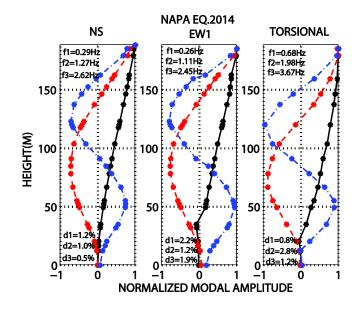
*Figure 6.* Three mode shapes and associated modal frequencies and damping percentages extracted from NS, EW and Torsional acceleration.
