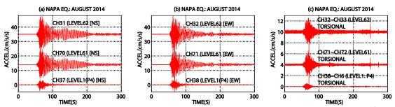
*Figure 5.* Equiscaled (a) NS, (b) EW and (c) torsional acceleration time-history plots each for  $61^{st}$ ,  $62^{nd}$  and  $1^{st}$  levels. Note the beating effect at  $61^{st}$  and  $62^{nd}$  floor accelerations in the NS and EW directions.
