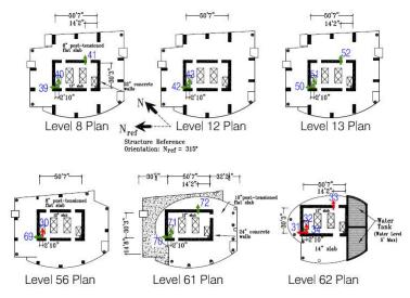
*Figure 2.* Typical plan views exhibiting sensor locations (green and red arrows), general dimensions and the core shear wall and outrigger columns (<u>www.stongmotioncenter.org</u>, last visited July 29, 2012). Note the building north reference direction ( $N_{ref}$ ), which is termed NS in this paper. The thickness of core shear wall is 32" between Level 1 and 32, 28" between Level 32 and level 55 and 24" between Level 55 and Level 64 (Roof).
