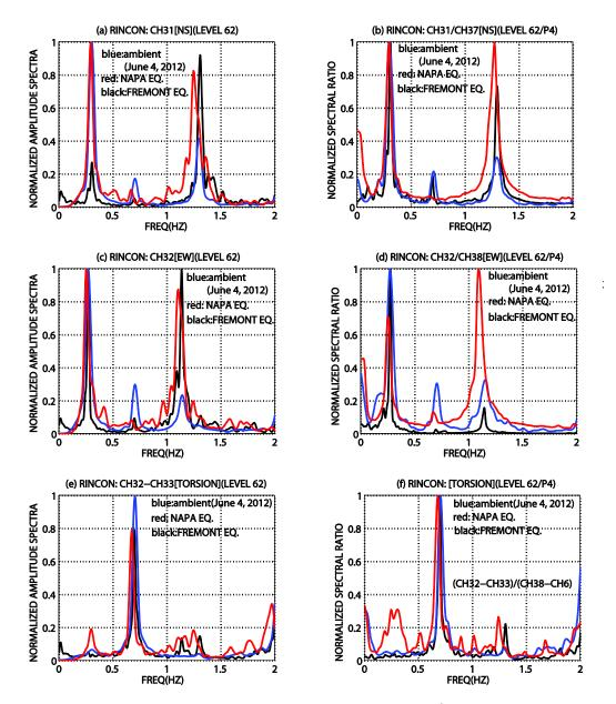
*Figure* 7. Comparison of 0-2Hz band normalized amplitude spectra from  $62^{nd}$  level accelerations (a) NS[CH31], (c) EW[CH32] and (e) Torsional [CH32-CH33] and normalized spectral ratios from amplitude spectra of  $62^{nd}$  and  $1^{st}$  (P4) level accelerations (b) NS[CH31/CH37], (d) EW[CH32/CH38] and (f) Torsional [(CH32-CH33)/(CH38-CH6)].
