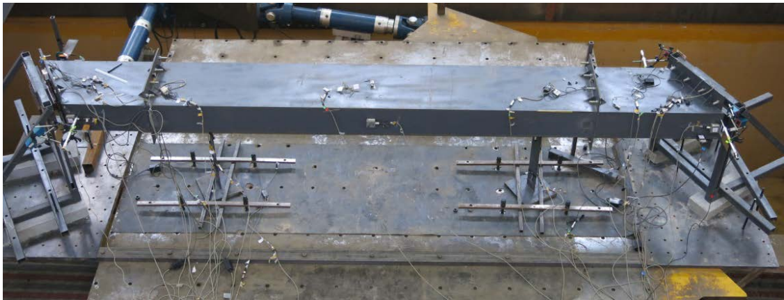
Figure 2: Setup of 30° skewed bridge on shake table
