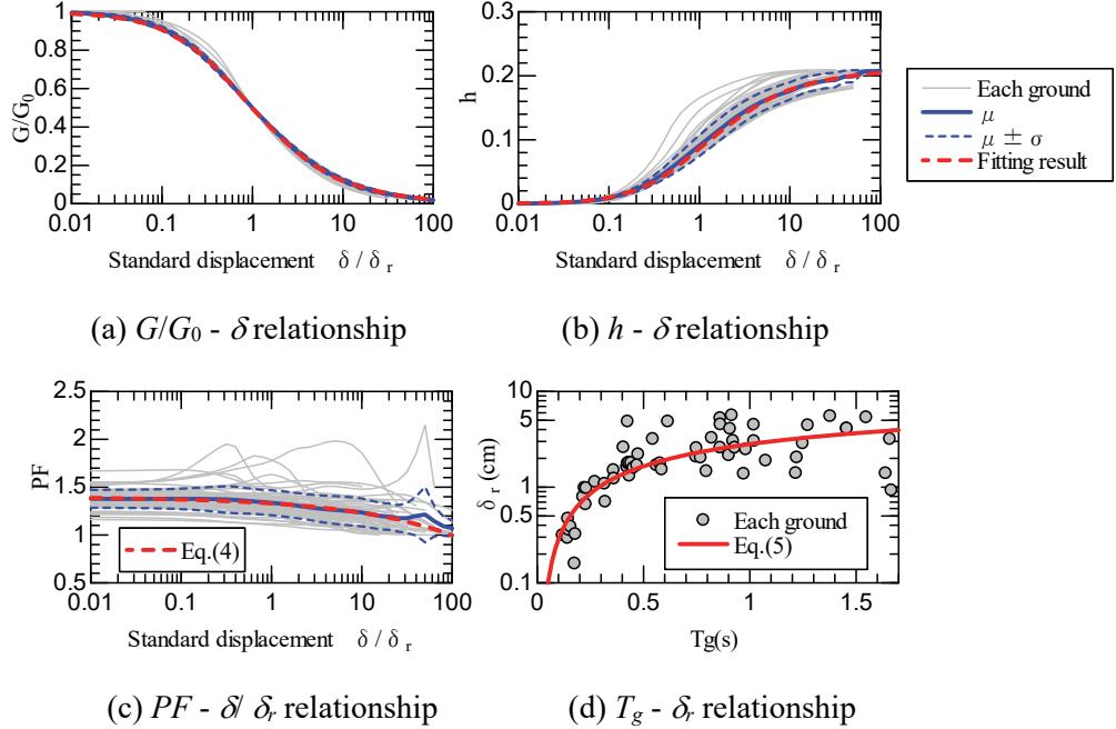
Fig. 3 Results of the static non-linear analysis after normalization using reference displacement  $\delta_r$
