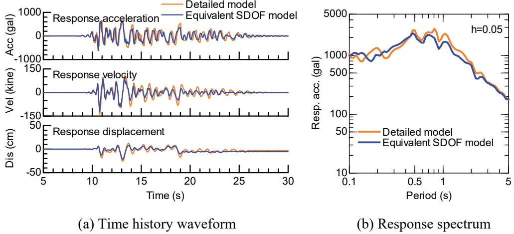
Fig. 5 Results of the prediction of the ground surface waveform by using only the natural period  $T_g$
