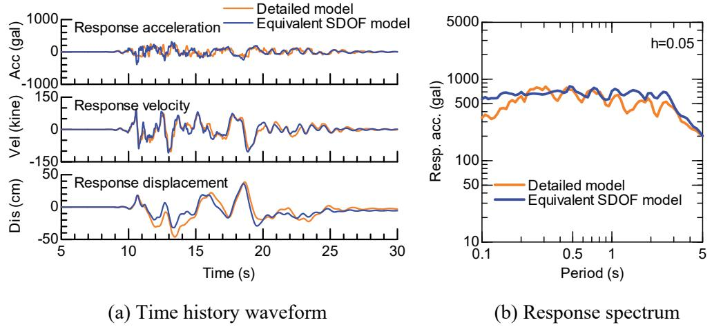
Fig. 6 Results of the prediction of the ground surface waveform by using only the natural period  $T_g$
