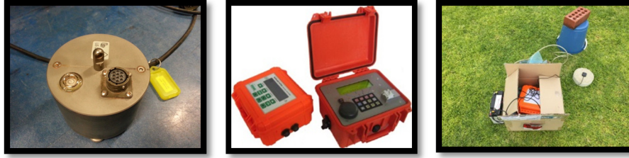
Figure 1. HVSr technique main equipment and data acquisition setup
