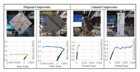
Fig 2. Prism failure modes and stress-strain curves
