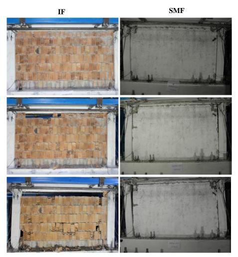
Fig 7. Infill panel damage of IF and SMF at 0.5%, 2% and 4% drift ratios
