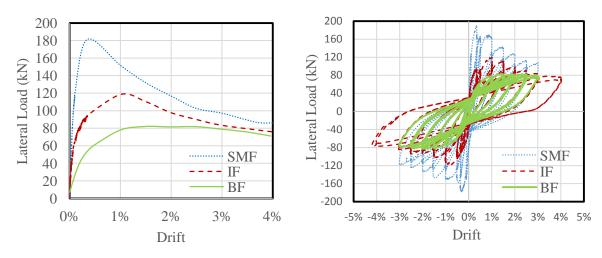
Fig 8 Backbone curves and hysteretic responses of tested frames
