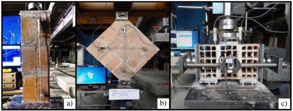
Fig 1. Prism tests; a) uniaxial compression, b) diagonal compression, c) split tension
