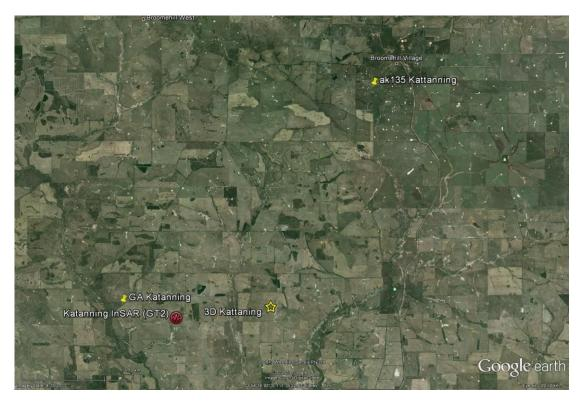
Figure 3. Katanning: This mb4.0 earthquake was accurately located using InSAR surface deformation measurements. Location errors are d(ak135)=14.0 km, d(3D)=4.4 km and d(GA)=2.6 km.
