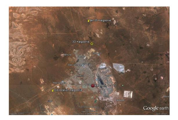
Figure 4. Kalgoorlie: This mb5.0 earthquake was well located using a local mine monitoring network. Location errors are d(ak135)=12.6 km, d(3D)=8.3 km and d(GA)=8.3 km. Using only P and S phases on 7 stations < 6 degrees distant this improves to d(ak135)=9.6 km and d(3D)=4.5 km.
