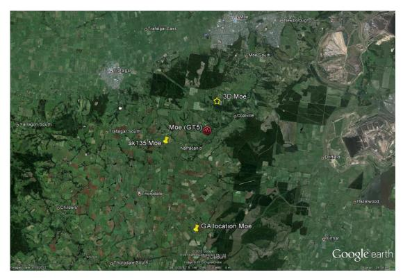
Figure 7. Moe. This Mw5.4 earthquake was well located using a regional network (Dan Sandiford, pers. comm.). Location errors are d(ak135)=3.3 km, d(3D)=2.3 km and d(GA)=7.5 km. S phases were difficult to pick for this event.
