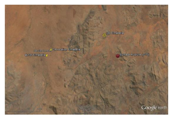
Figure 5. Ernabella: For this Mw5.3 earthquake ground truth was obtained using an observed surface rupture. Location errors are d(ak135)=14.2 km, d(3D)=4.8 km and d(GA)=13.4 km.
