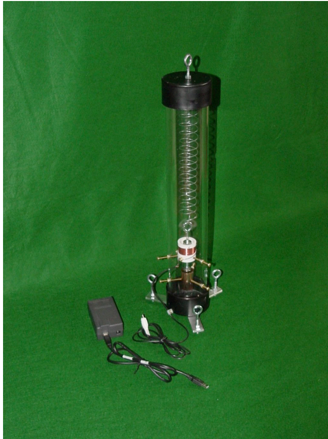
Figure 5. Slinky Seismometer developed by Boise State University (see http://cgiss.boisestate.edu/bsu-network/ )
