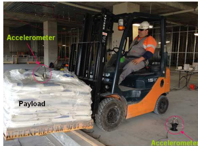
Figure 2: Fork-lift up/down test (accelerometer on back of forklift is invisible)
