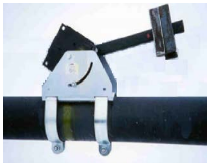
Fig. 2. A photo of an installed TMD on a pipeline
