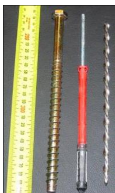
(b) The three retrofit cavity ties used in Auc-W1B, Auc-W2, and Auc-W3, respectively (left to right)
