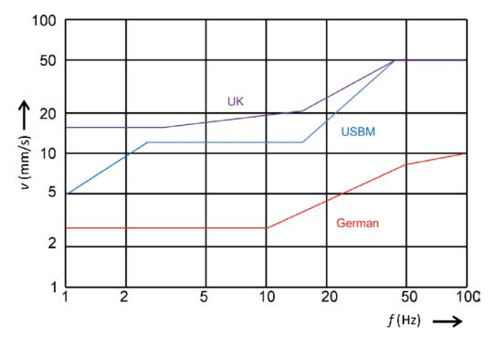
Figure 1: Comparison of frequencies v. PPV for some commonly quoted standards
