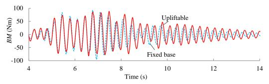
Figure 2: Effect of uplift on the bending moment
