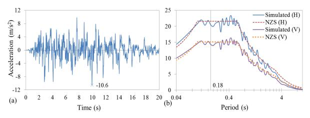
Figure 3. (a) Simulated ground acceleration in horizontal direction and (b) acceleration spectra of simulated excitations in both directions with 5% damping
