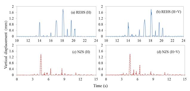
Figure 5. Vertical displacement of footing under the REHS and NZS motions (a)(c) without and (b)(d) with vertical component
