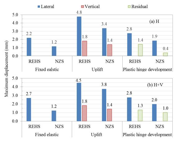
Figure 4. Maximum lateral, vertical and residual out-of-plane displacements of the bridge (a) without and (b) with vertical excitation
