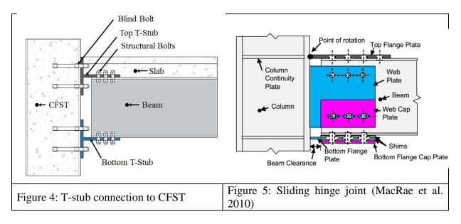
If the beam rotates about the top corner of beam, unlike the T-Stub yielding case, the reinforcement within the slab will not be activated. Thus, the capacity of composite beam near the connection (in the hogging region) decreases and larger sections are required to meet the demand. Col 4 of Table 1 shows the section sizes required for such case.
