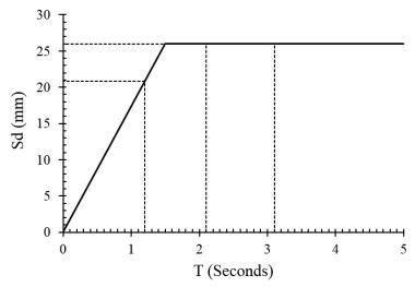
Figure 3: Elastic displacement response spectra
