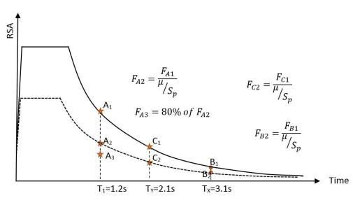
Figure 2: Acceleration Response Spectra where  $T_1$  is from AS 1170.4:2007,  $T_X$  and  $T_Y$  are modal periods in the X and Y directions respectively (figure not to scale).
