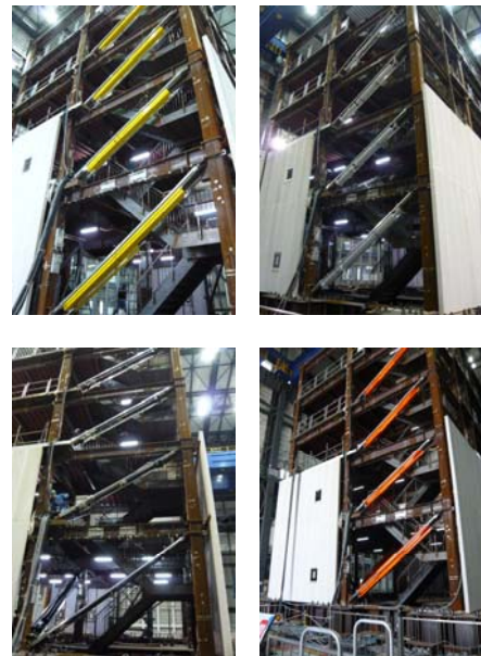
Figure 3 Four Types of Dampers in Building Specimen (View of Exterior Frame)
