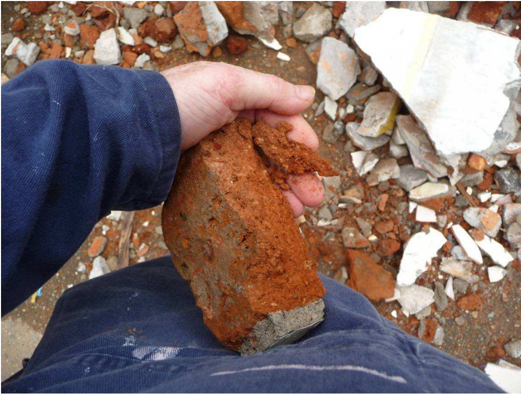
Figure 6 Soft bricks--Broken with fingers
