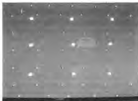
Figure 3: Targets on 'calibration wall' illuminated by flash.
