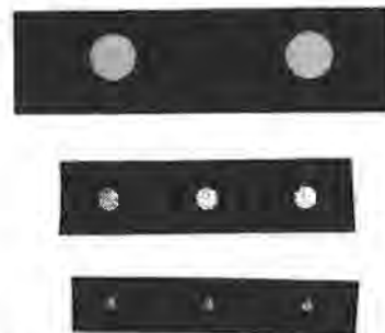
Figure 2: Retro-reflective targets 12mm, 6mm and 3mm in diameter.
