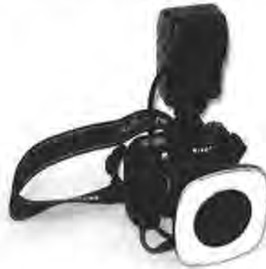
Figure 1: Nikon D100 with Sunpak ringflash and optical stabilisation.
