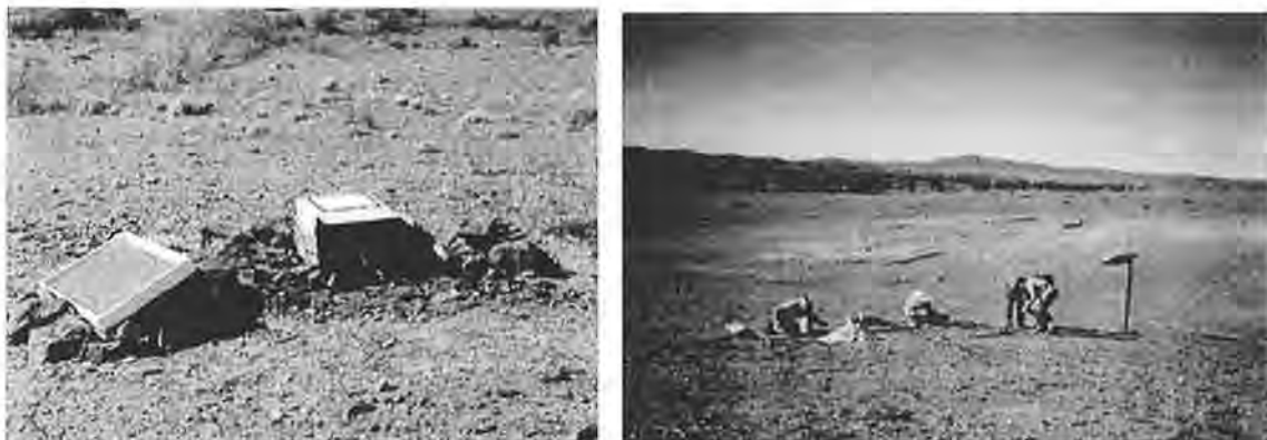
Figure 1. Comparison of deployment styles for Kelunji (left, station FR03) and Reftek (right, station FR05) equipment. Both sites are east of Hawker, SA, near the eastern margin of the Flinders Ranges. Seismometers are buried in either case.
