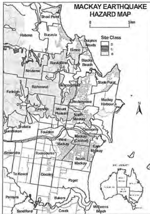
Figure 1: Earthquake hazard map for Mackay. Rock (Site Class B) outcrops in the northwest of the map. Site Class C is a small area of hard sediments. Large areas of Mackay are underlain by alluvial and marine sediments (Site Class D)
