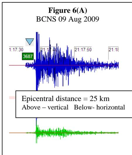
Earthquakes of about 2 km depth or less commonly have a well-developed *R<sub>g</sub>* phase seen at the more distant stations. Typical seismograms for Beacon events (in this case 09 Aug 2009, ML 2.7) from BCNS and MORW are reproduced here (**Figure 6 A&B**). *R<sub>g</sub>* phases are not apparent on these seismograms, and McCue (pers comm., 2009) suggests on the basis of these observations that the events probably have depths of approximately 5 km or greater.
