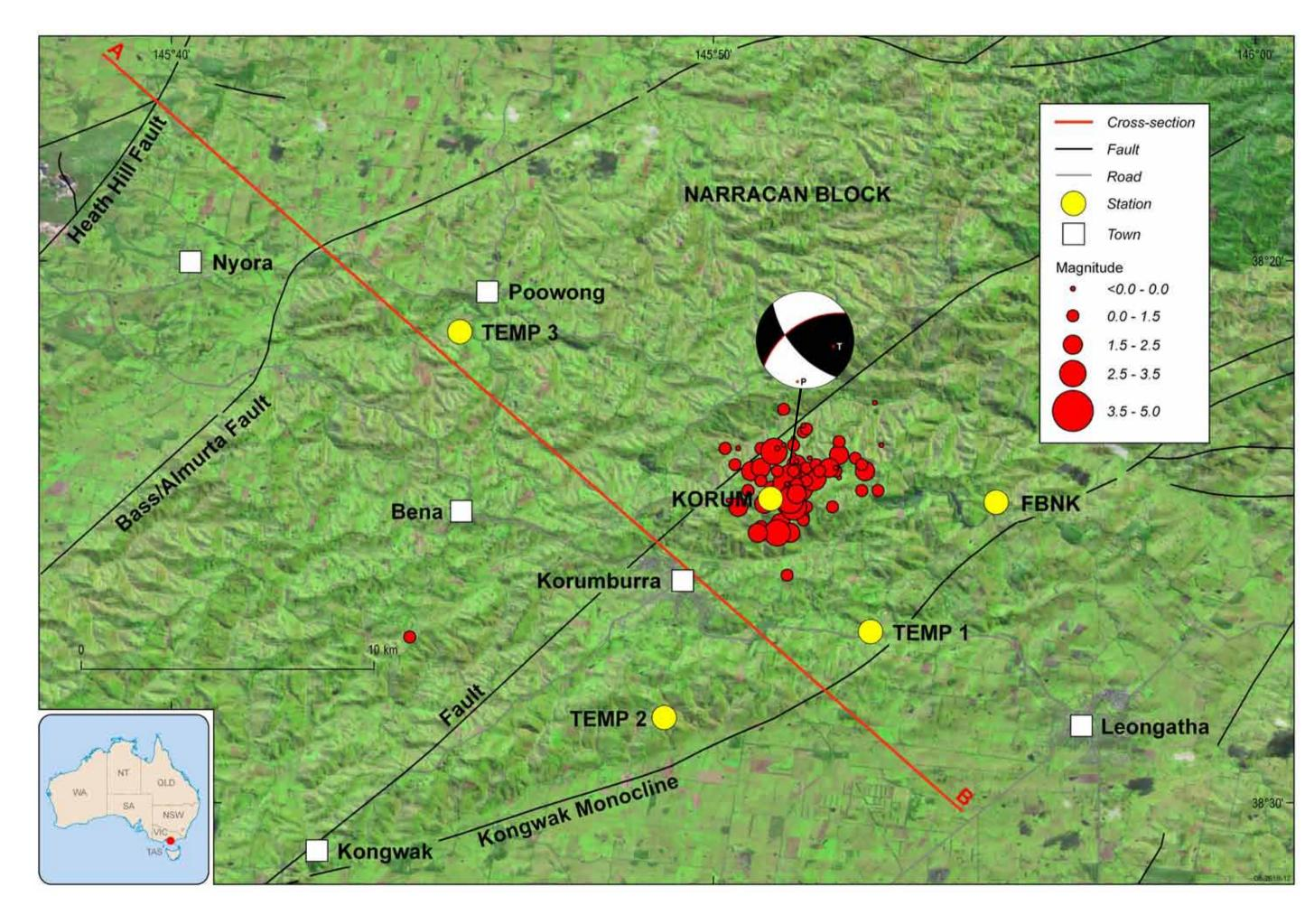
Figure 1. Plot of epicentres of the March 2009 Korumburra earthquakes, and temporary seismographs, overlaid onto the 3-second SRTM DEM data with major fault traces marked. Focal mechanism courtesy of Kevin McCue (preferred nodal plane marked). A-B marks the cross section shown in Figure 2.
