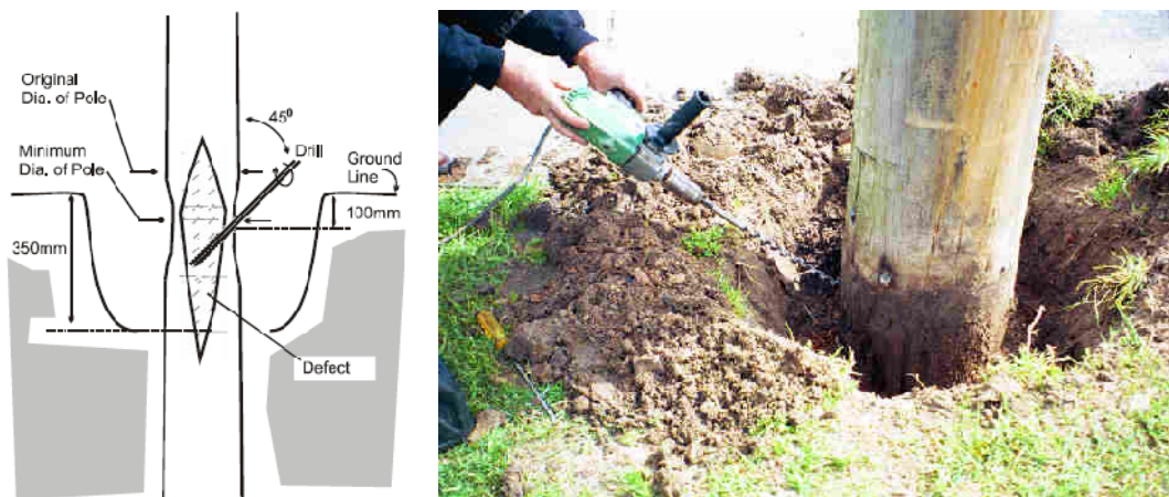
Figure 3: Details of inspection below ground line
