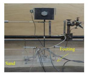
Figure 3. Shake table test setup
