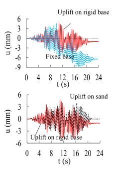
Figure 4 (above). Effect of uplift and support flexibility on structural response
