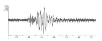
The above accelerogram is from a JUMP recorder (GHS) installed a few blocks away. The equipment is a triggered Kelunji Classic KA1 with a Guralp CMG-5T accelerometer. The vertical component is shown above. The P wave is visible from just before 12 seconds, and the ground roll (surface wave) is very clear from 13.5 seconds. 2,000,000 counts is approximately 1g.
