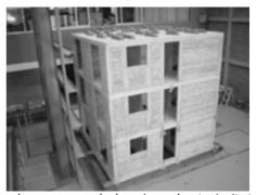
Replica houses are shaken in order to imitate earthquakes. *Courtesy of UNAM*
