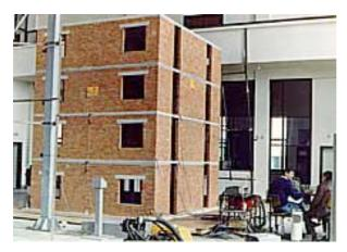
**Figure 2** Modelling of Mixed Reinforced Concrete Masonry Buildings at IZIIS Macedonia (joint program with Istituto di Tecnica Delle Costrucioni, Universita di Bologna, Italy
