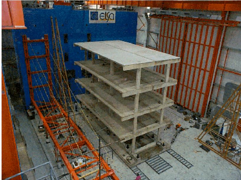
**Fig. 1** – Test frames prior to testing at Joint Research Centre, Ispra, Italy
