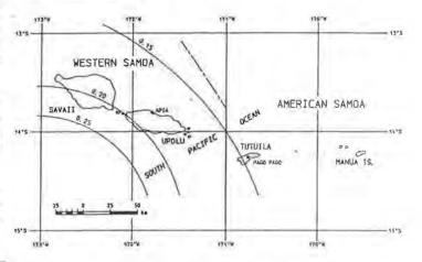
Figure 3 Acceleration Coefficient Contours for Samoa (500 year average recurrence interval)
